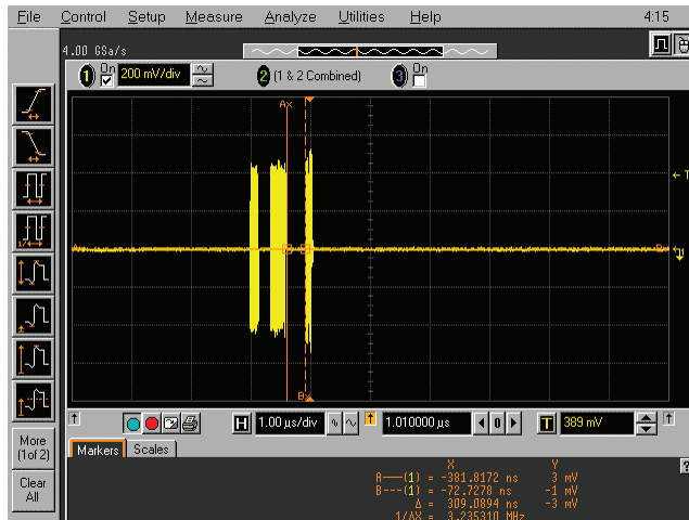
Figure 13. Device inter-packet gap.
