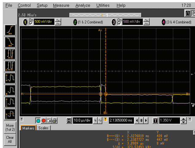
Figure 16. Time between last J in CHIRP and high-speed termination initiation.
